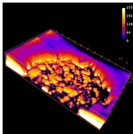
Figure 5. The contact area 3D image between PS bead and the glass coverslip. Size 80 × 80 μm.
