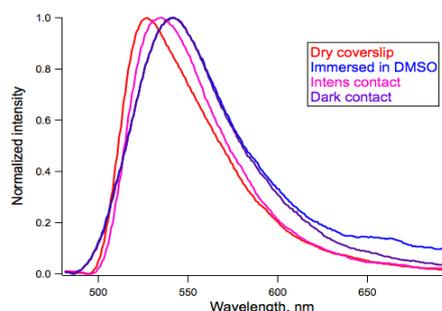
Figure 2. Spectra of the compound 1 immobilized on coverslide in contact with PMMA bead and immersed in solvent.
