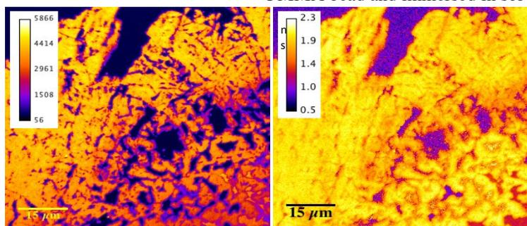
Figure 3. Contact area fluorescence intensity image versus fluorescence lifetime image between PMMA bead and the glass coverslip with a monolayer of compound 1. Relatively short lifetimes in the "dark contact" regions indicate presence of the solvent in the area.
