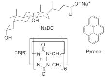
The gel network is formed from NaDC aggregates, but some of these aggregates remain soluble in the trapped aqueous phase of the gel. Pyrene was used as a fluorescent probe molecule, which is hydrophobic and is solubilized within the gel. Cucurbit[6]uril (CB[6]), a macrocyclic host, was added to mechanically strengthen the gel and also served as a host for the weak binding of pyrene. Steady-state and time-resolved fluorescence studies showed that at low temperatures pyrene was located in the
